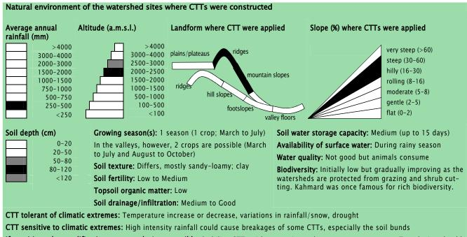
**If sensitive, what modifications were made / are possible:** Stabilize CTTs with vegetative and management measures. Trench size should be based on hydro-meteorological parameters considering possibility of an extreme event occurring.
