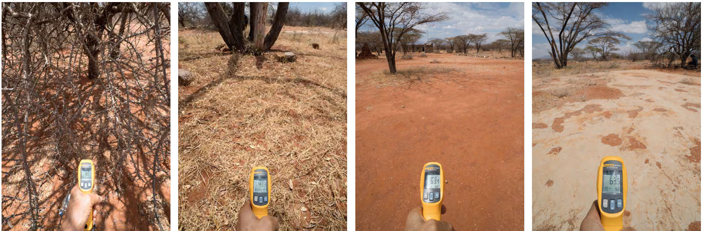
Figure 2: Early afternoon soil surface temperature in the northern Kenya semi-arid lowlands. From left to right: (a) 50% dry bush/ grass cover = 33°C (b) 50% dry grass cover = 43°C (c) on bare soil = 63°C and (d) on bare gneiss rock = 63°C (Hanspeter Liniger).
